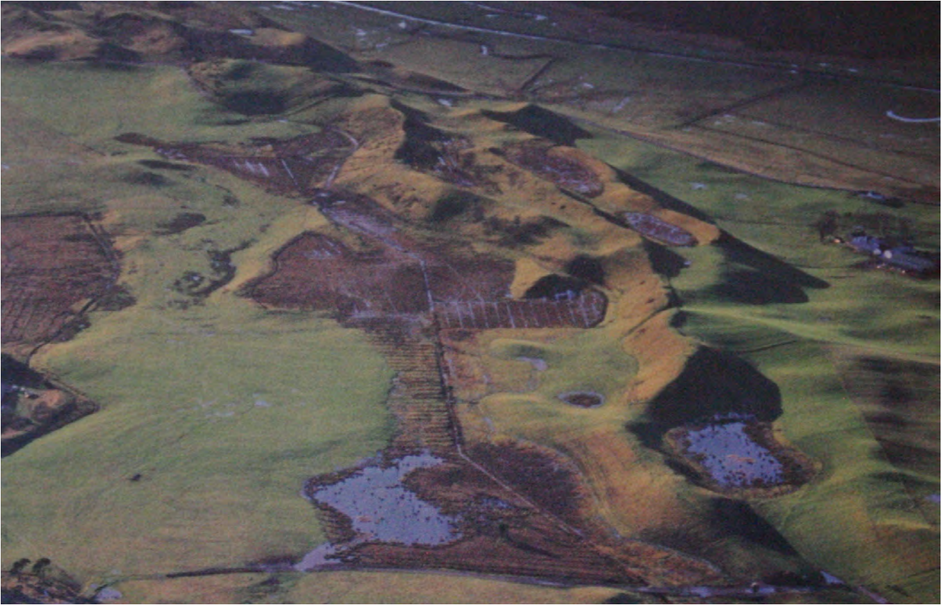
Photo 3.5. Sand and gravel extraction from a protected Ice Age esker in Scotland has permanently destroyed the integrity of the landform. © P & A Macdonald/SNH
